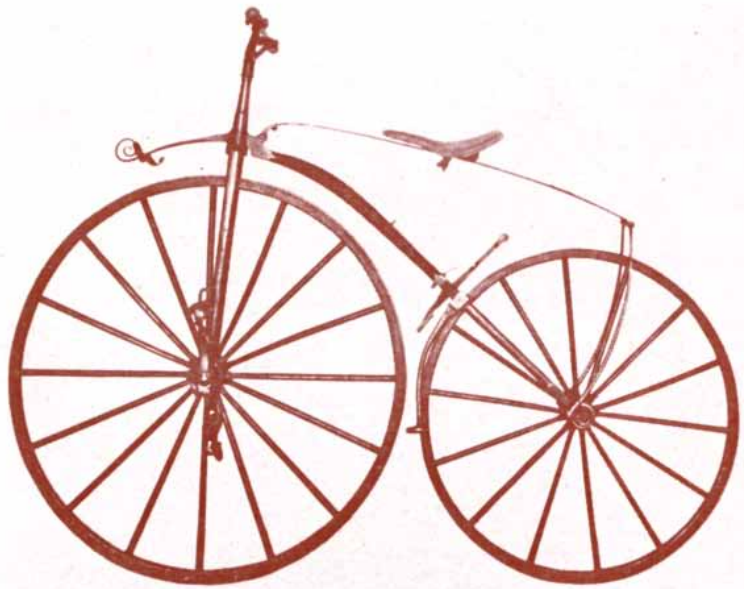
FRENCH VELOCIPEDE , produced by Pierre and Ernest Michaux in Paris in 1863, was the first commercially important machine on the way to the modern bicycle. The "bone-shaker," as the vehicle was sometimes called, had cranks with pedals fixed directly to the hub of the front wheel and hence suffered from the limitation of having too low a gear ratio.
